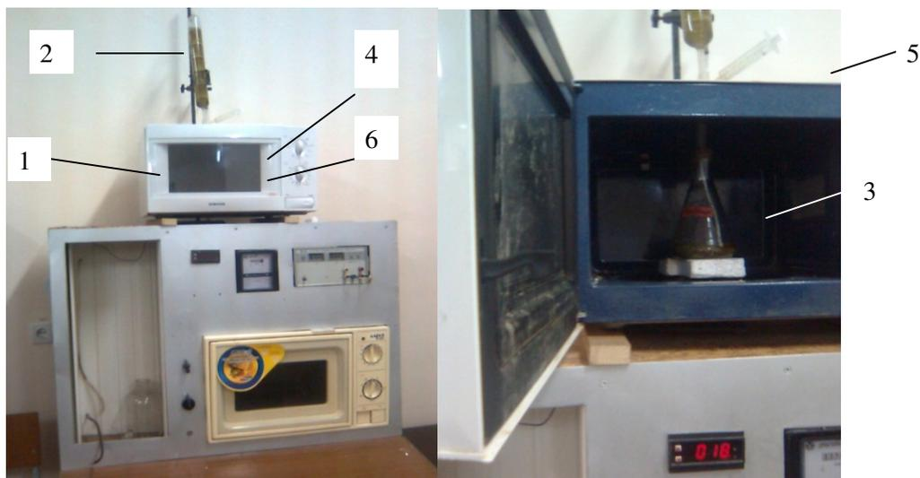
Fig. 1. **Stand for oil extraction:** 1 – high-frequency microwave camera; 2 – reverse water cooler; 3 – chamber with the product; 4 – power control; 5 – syringe for taking samples; 6 – timer
