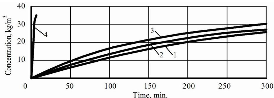
Fig. 3. **Dependence of concentration on time in the process of extraction of oilcake by alcohol (colza + alcohol, oilcake 2-4 mm, 1: 3, no MW) at different temperatures:**
