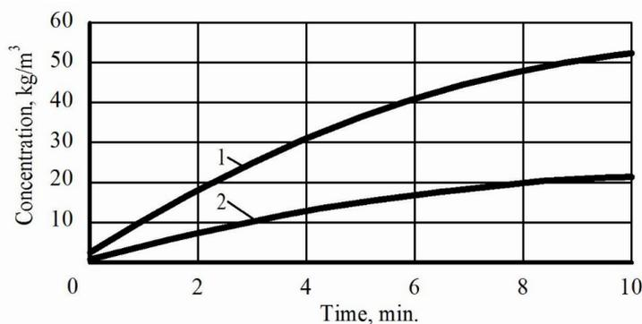
**Fig. 9. Influence of the power of the microwave field in the process of extracting canola (colza + alcohol, corn 0.5-1 mm, 1: 3, 10 min, 78.3 °C) with alcohol:** 1 – MW; 2 –no MW.
