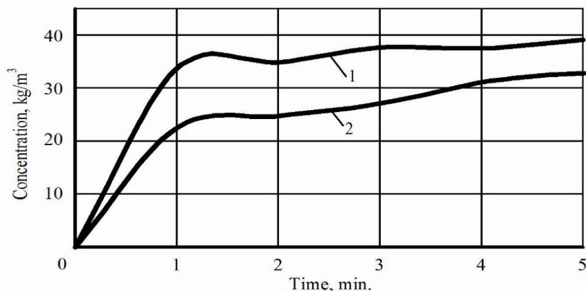
**Fig. 7. Effect of solvent during extraction of crushed canola seed meal with hexane and alcohol (oilcake 2-4 mm, 1: 3, no MW) without the influence of the MB field:**
