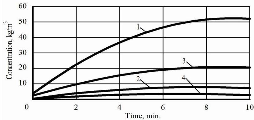
Fig. 4. Dependence of concentration on time in the process of extracting canola meal with hexane (colza + hexane, oilcake 2-4 mm, 10 min, MW) at various ratios of solid and liquid phases: 1 – 1: 3; 2 – 1: 20; 3 – 1: 10; 4 – 1: 5.
