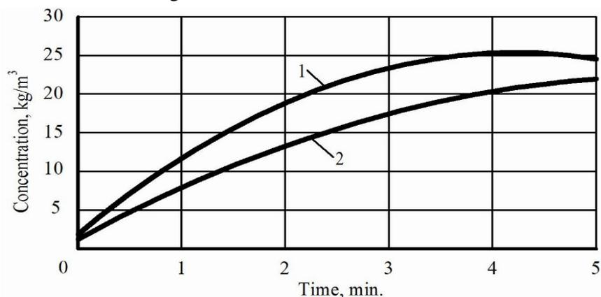
Fig. 6. Influence of the solvent in the process of extraction of crushed grain of canola seeds with hexane and alcohol (corn 0.5-1 mm, 1: 3, no MW, 5 min) without the influence of the MB field: 1 – colza + hexane, 68.7 °C; 2 – colza + alcohol, 78.3 °C
