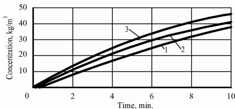
Fig. 11 Influence of the power of the microwave field in the process of extracting oil from canola meal (colza + alcohol, oilcake 2-4 mm, 1: 3, MW, 10 min, 78.3 °C) with alcohol: 1 – 127 W; 2 – 255 W; 3 – 425 W
