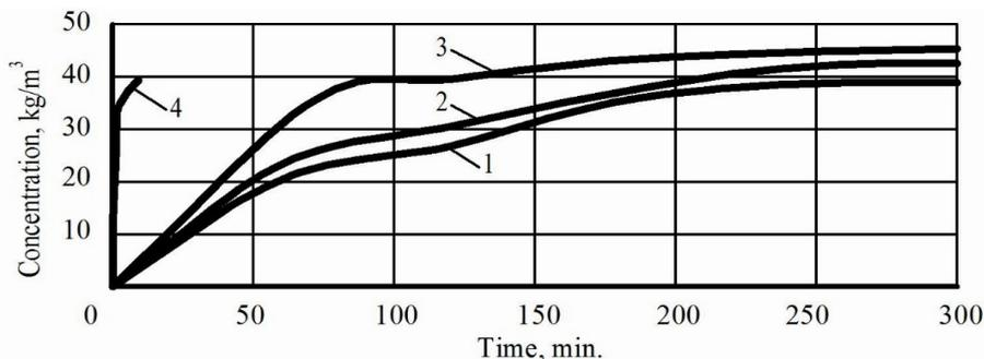
Fig. 2. **Dependence of concentration on time in the process of extracting canola seed meal with hexane (colza + hexane, oilcake 2-4 mm, 1: 3, no MW) at different temperatures:**
