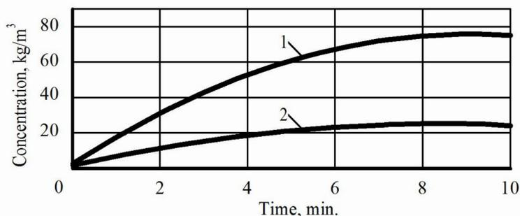
**Fig. 8. Influence of the power of the microwave field in the process of extracting canola seeds (colza + hexane, corn 0.5-1 mm, 1: 3, 10 min, 68.7 °C) with hexane:**
