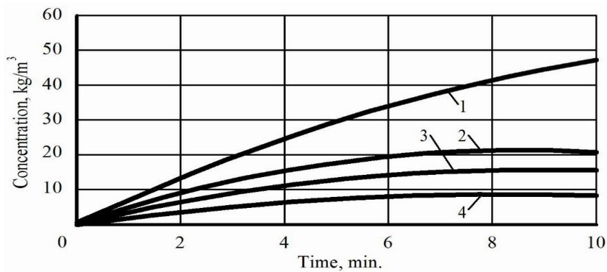
Fig. 5. Dependence of concentration on time in the process of extraction of oilseed meal with alcohol (colza + alcohol, oilcake 2-4 mm, MW, 10 min, 78.3 °C) for various ratios of solid and liquid phases: 1 – 1: 3; 2 – 1: 5; 3 – 1:10; 4 – 1:20
