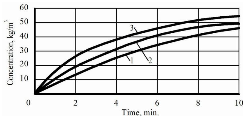
Fig. 10. Influence of the power of the microwave field during extraction of oil from canola meal (colza + hexane, oilcake 2-4 mm, 1: 3, MW, 10 min, 68.7 °C) with hexane: 1 – 127 W; 2 – 255 W; 3 – 425 W
